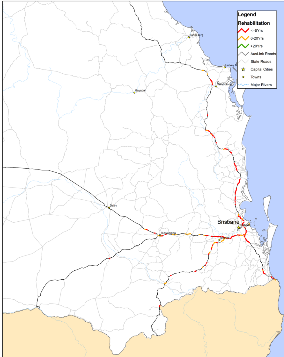
AusLink - Surface condition and deflection triggered additional rehabilitation works
